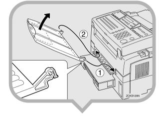
**3.** Hold the Document Delivery Tray at the points indicated by the circles in the illustration, then attach it to the fax machine. Attach the Document Delivery Tray.
